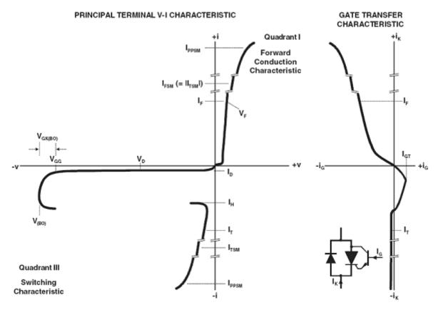
SVG170Q Principal Terminal and Gate Transfer Characteristics
